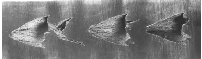
Fig. 8. End cavities in section of leaded brass rod (Bauser, 2006).
