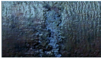
Fig. 1. Zinc segregates on brass CuZn40Pb2 billet (PERNIS, 2011).
