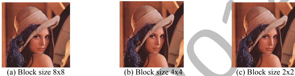
Figure 6 : Decompressed Image Of Lena For Block Size 8x8, 4x4 And 2x2 Using The Proposed GA Technique.
