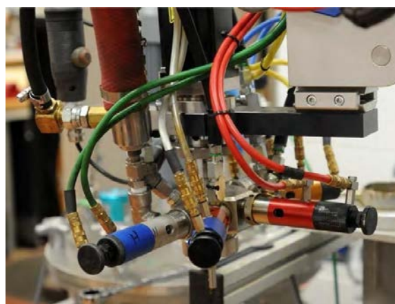
Figure 2: Dynamic mix head with valves
