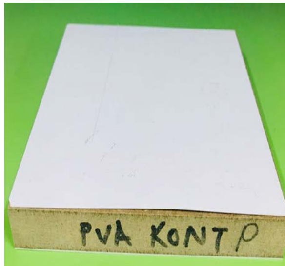
Figure 12. Control sample: PCV veneer bonded with PVAc adhesive
