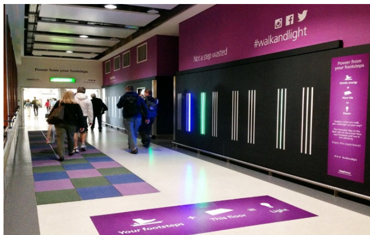
Figure 1. UK-based Pavegen company makes electricity-generating flooring ( www.futureentech.com/2016/05/pavegens-power-generating-floor )
