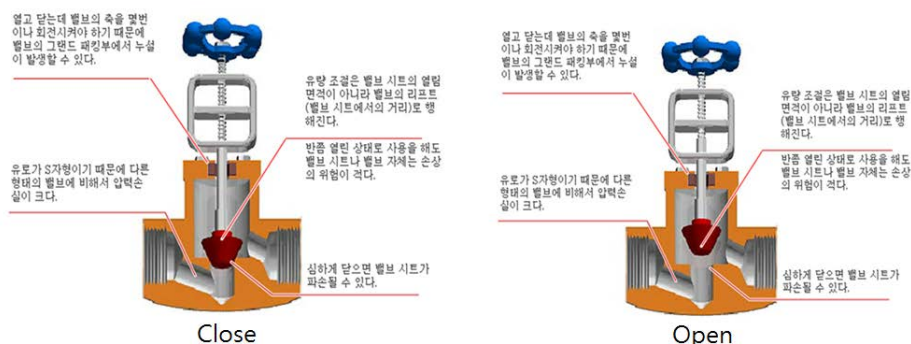
Figure 3. Structure and Operation of Globe Valve
