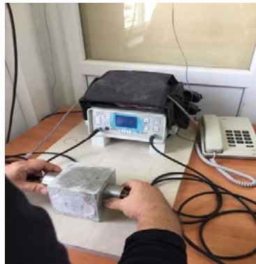
Figure 3. Ultrasonic measuring instrument
